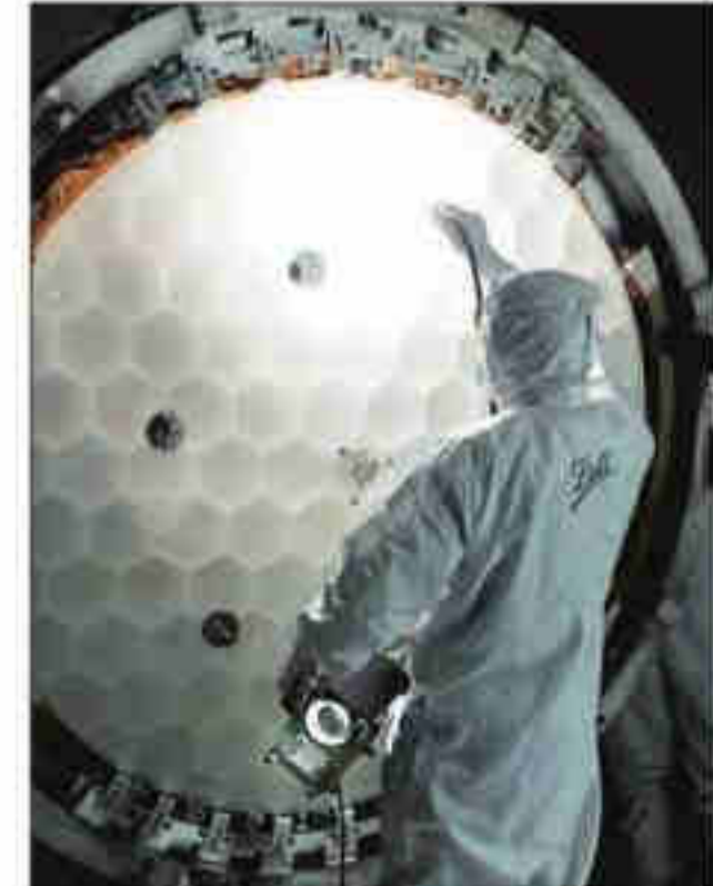
Technicians inspect the back of the Kepler telescope's primary mirror. Ball Aerospace via The New York Times
